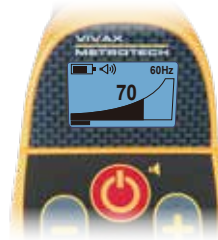
Peak locate response with accompanying audio tone
