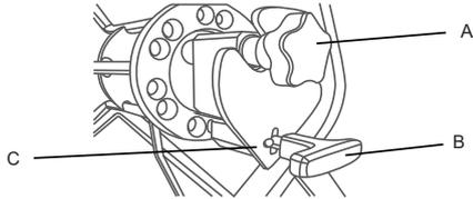
**Cable Guide** - Turn the reel so that the pushrod goes through the cable guide.
