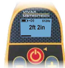
Push button depth reading
