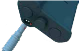
Battery charging port and charger plug
